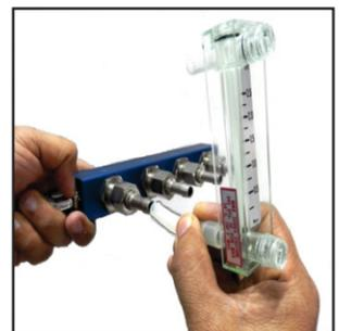
Fig. 3: Connecting flow meter to manifold port
