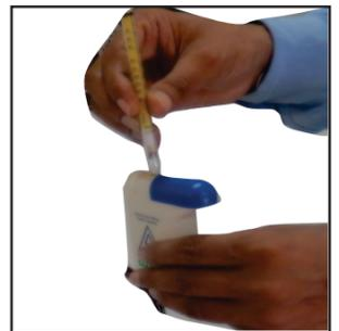
Fig. 5: Breaking off detector tube tips
